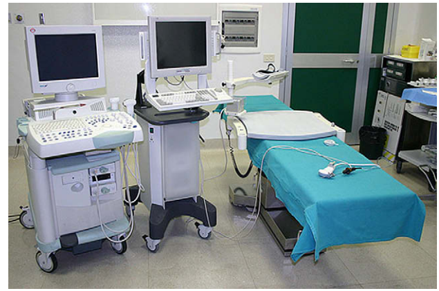
Figure 1 The Navigator system ® (from left to right): ultrasound scanner, TECHNOS MPX. Navigator System ® (with touch-screen monitor) connected to the navigation system, which consists of a passive electromechanical sensor (near the patient) and an active sensor attached to the ultrasound probe.
