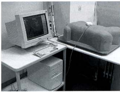
Fig. 3 The ultrasound simulator, consisting of a powerful computer, a life-like mannequin with an integrated electromagnetic localisation unit and a 3-dimensional sensor inside the dummy transducer.
