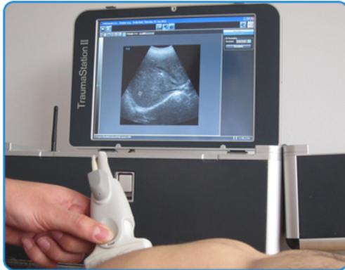
A technician uses the TraumaStation II to take an ultrasound scan. Ascension's 3D Guidance driveBAY sensor is mounted on the back of the ultrasound probe. Both parts are precisely calibrated, enabling Ascension's tracking system to record the local position and orientation of the ultrasound probe while the ultrasound image is acquired. With the aid of the sensor, TraumaStation II is able to generate 3D volumes from 2D ultrasound sequences.
